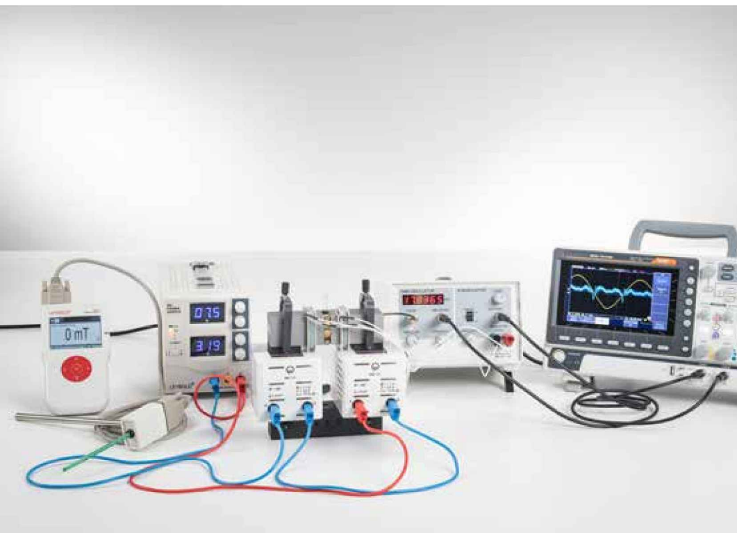
Nuclear magnetic resonance (NMR) on water, polystyrene, glycerine and Teflon (C3.4.3.1)
